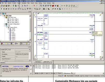
Ladder Diagram Editor provides a display of the PLC application, and indicates the Off-line and On-line values of application variables. Force status for discrete variables and Retentive status for coils is also indicated.
