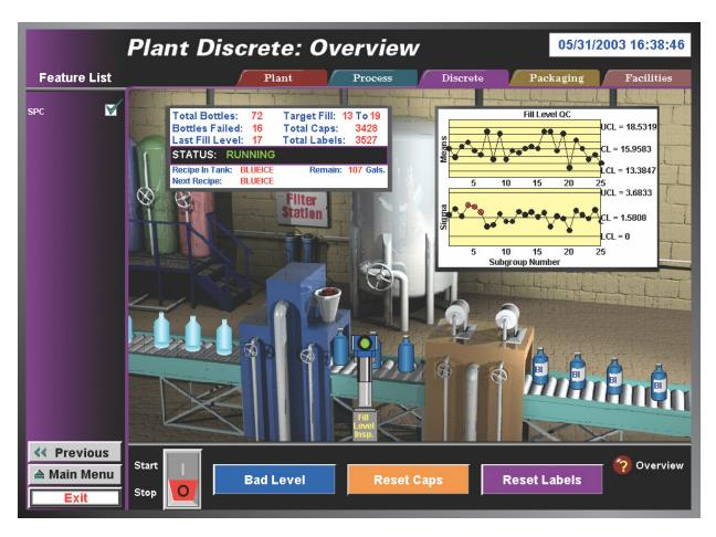
CIMPLICITY HMI can be enhanced with powerful option modules such as SPC that are fully integrated. Your operations can be monitored continuously and any SPC related alarms are handled with the same common alarm viewer.
