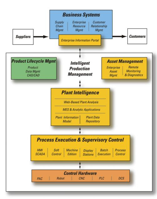
Intelligent Production Management (IPM) integrates all key areas of the production management lifecycle, giving you greater connectivity, analysis and control over your operation. **CIMPLICITY HMI** is part of GE Fanuc's **Process Execution & Supervisory Control** family of IPM solutions.
