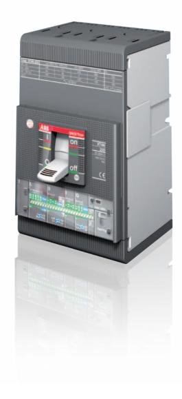
In marine applications, for example, high breaking capacities at 690V are required. The SACE Tmax XT2 and XT4 circuit-breakers reach the highest breaking capacities on the market. In particular, XT2 has an Icu of 20kA@690V, 150 kA@415V whereas XT4 reaches an Icu of 90kA@690V for 160A, 150kA@415V for 250A.
